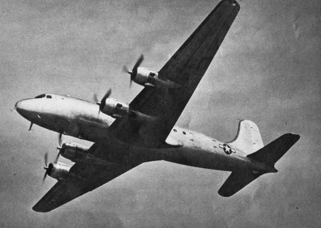
C-54'S NOSE PROJECTS WELL BEYOND EQUALLY TAPERED WING. TAILPLANE HAS ROUNDED TIPS
